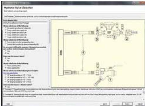
PDS (Package Design Software) is an interactive tool designed to configure coil-piping packages and hose kits. This real time, step by step drawing tool drastically streamlines the take-off and order process by simultaneously creating a drawing, quotation and spec submittal, all through a simple point and click application.
